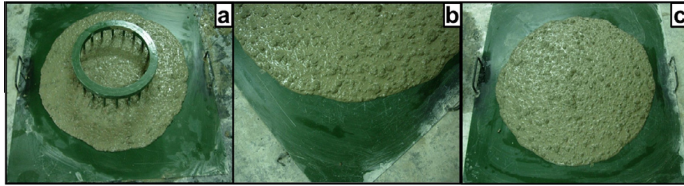
Fig. 3. Tests in the fresh state. a. Sample SRG after the J-ring test, b. Edge of sample HRGF after the extended test, c. Extended test of sample HRGF.
