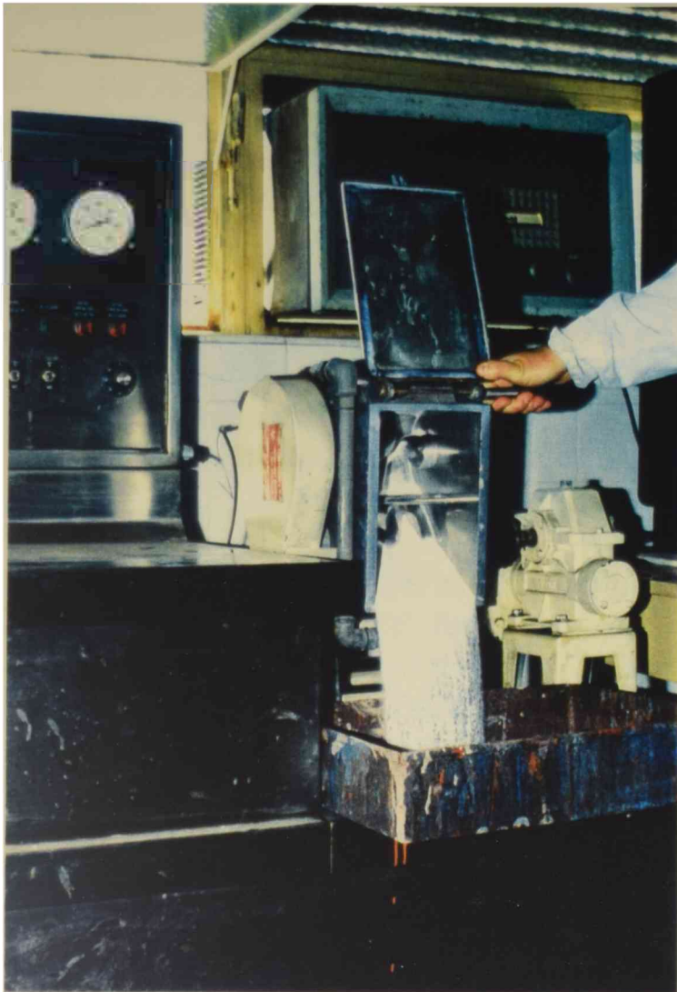
Fig. 1.- Double Z mixer for test samples preparation.
