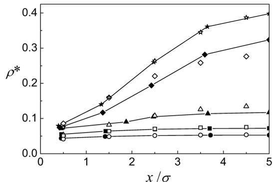
Figure 1: Density profiles for a  $n=9$  layer model of a confined fluid in a slit pore (solid symbols). The temperature is  $T^*=1.0$  and the wall separation is  $L=10\sigma$ , with mean densities  $\rho^*=1/20$  (circles),  $1/15$  (squares),  $1/10$  (triangles),  $1/5$  (diamonds), and  $1/4$  (stars). Open symbols represent the Monte Carlo simulations.
