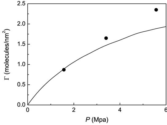
Figure 5: Excess number of molecules per unit area of pore surface  $\Gamma$  as function of the external pressure. The full line represents the experiment (digitalized from Ref. [19]), and the dots are our theoretical results.
