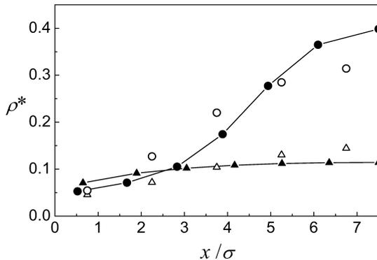
Figure 3: Density profiles for a  $n=13$  layer model of a confined fluid in a slit pore (solid symbols). The temperature is  $T^*=1.0$  and the wall separation is  $L=15\sigma$ , with mean densities  $\rho^*=1/10$  (triangles), and  $1/5$  (circles). Open symbols represent the Monte Carlo simulations.
