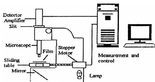
Figure 2. Schematic of the spectroscopic plate reading setup.
