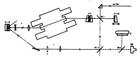
Fig.4 Intra-cavity phase conjugation experimental arrangement.
