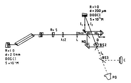
Fig. 1 Experimental arrangement for extra-cavity phase conjugation
