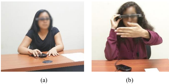
Figure 1. Participant in front of desk wearing smart glasses: (a) using Trackpad; (b) using gesture control
