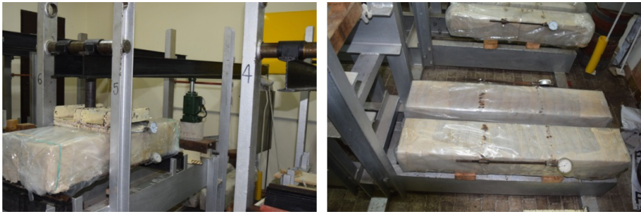
Fig. 2. Load RC beams (left) and reference unloaded ones (right).
