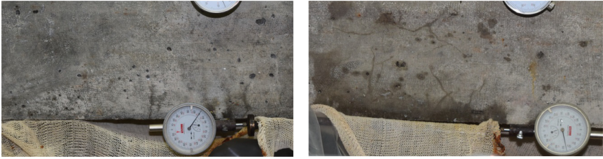
Fig. 7. Appearance of the surface of loaded R and FR beams at the age of 5 months.
