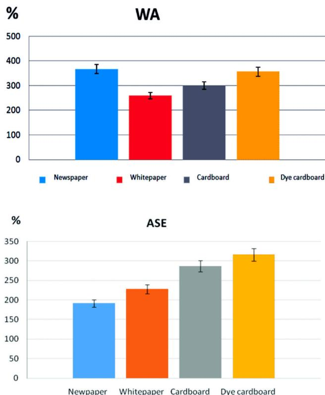
Fig. 3. Graph of WA, %, and Anti-shrink Efficiency (ASE, %) after soaking and drying cycles according to Rowell.
