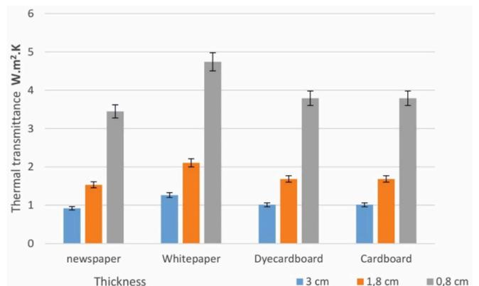
Fig. 9. Thermal transmittance (U).
