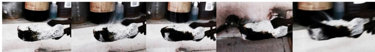
*Newspaper: Generates flame when exposed for duration of 10 seconds. The repellent of this may be observed until the last test (30 seconds) inclusive. The loss of the material is lower in relation to other materials.*
