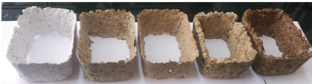
Fig. 2. Thermal and acoustic insulation test specimens: The different types and grosser of samples allowed measuring the isolation properties of material.
