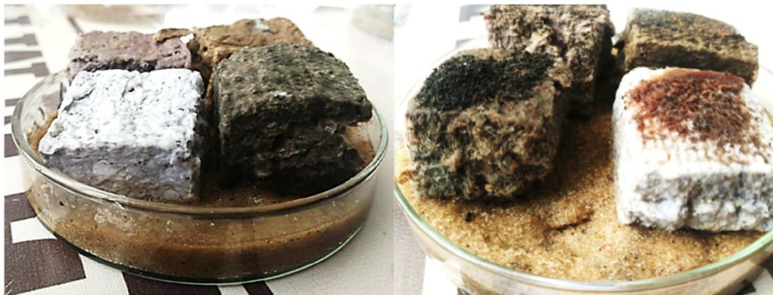
Fig. 6. It pictures panels without fungal inoculation (control) and inoculated for the study of biodegradation.
