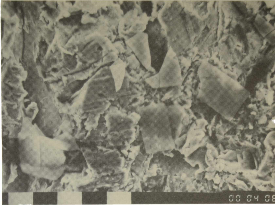
Fig. 11.- SEM micrograph of an uncoated steel surface obtained after removing the binder with trichlorethylene. Immersion time of the coated specimen: 24 hours in 0.5 M sodium perchlorate solution.
