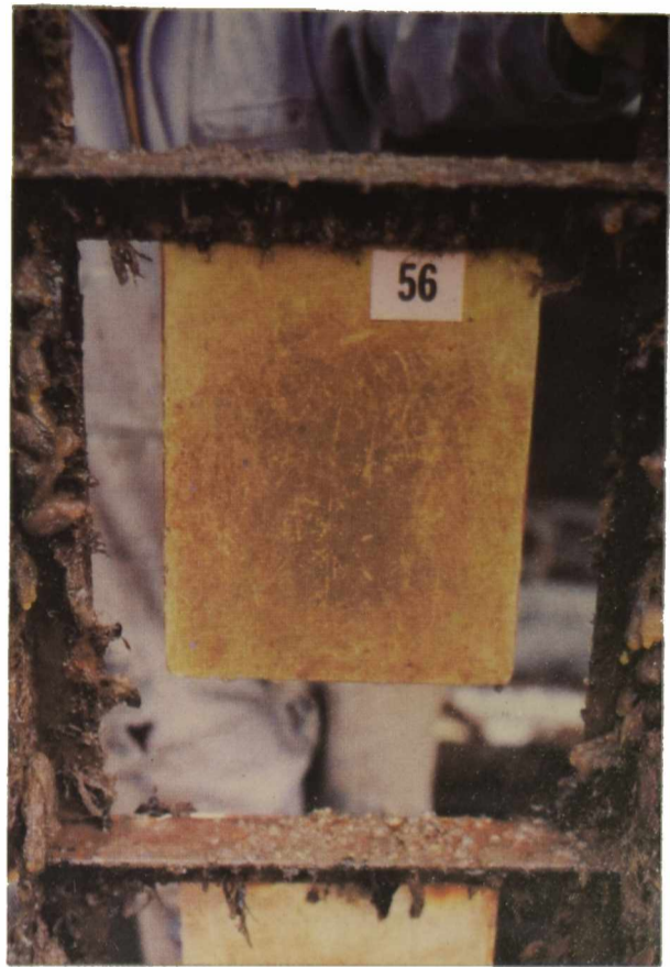
3.2. Disproportionated WW rosin Dry film thickness required, minimum 250 \mu\text{m} Efficiency, 90 %
