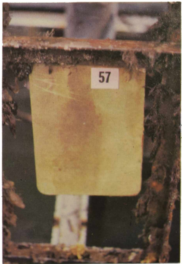
3.4. Disproportionated calcium resinate Dry film thickness required, minimum 200 \mu\text{m} Efficiency, 100 %
