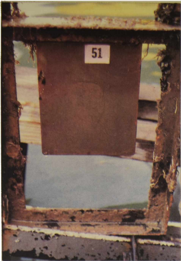
4.1. WW rosin resin Dry film thickness required, minimum 300 \mu\text{m} Efficiency, 100 %
