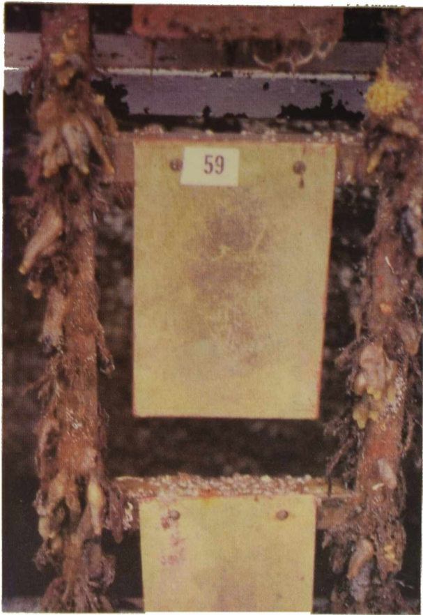
3.1. WW rosin resin Dry film thickness required, minimum 250 \mu\text{m} Efficiency, 100 %
