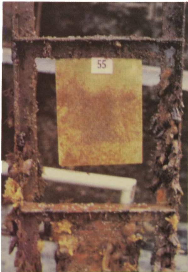
3.3. Calcium resinate Dry film thickness required, minimum 200 \mu\text{m} Efficiency, 90 %
