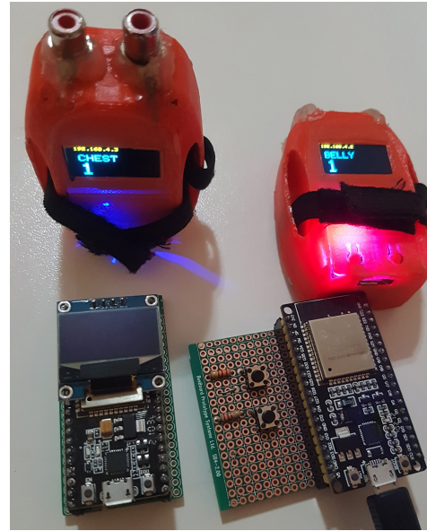
Figure 4: Voltaje divider circuit module with ESP32 micro-controller. Two multiclient modules and one server module.
