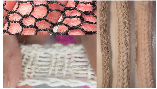
Figure 9: Different resistive yarn knit patterns used throughout the design iterations.
