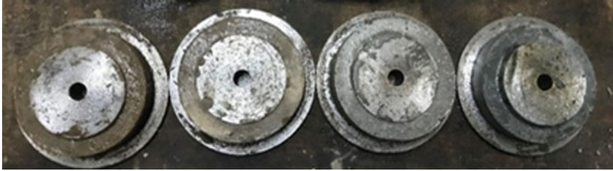
Fig. 3 Determination of restrained shrinkage in paste rings with the addition of illitic calcined clay
