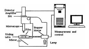
Figure 2. Schematic of the spectroscopic plate reading setup.
