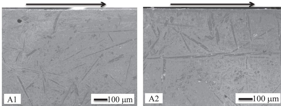
Fig. 12. Longitudinal section of A1 and A2 worn specimens.
