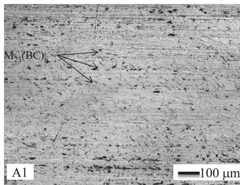
Fig. 11. SEM image of the A1 worn surface.
