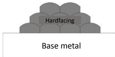
Fig. 1. Scheme of all weld metal coupon.
