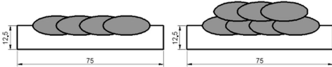
Fig. 2. Scheme of the coupons; units in mm.
