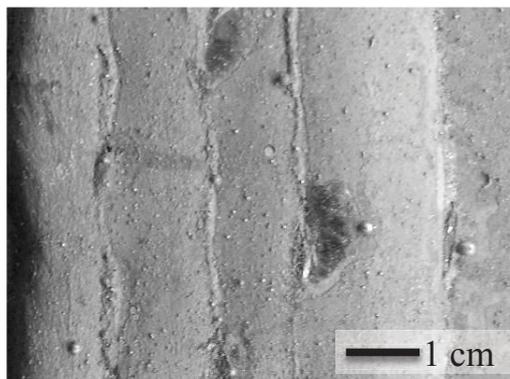
Fig. 4. Surface view of the welded beads.
